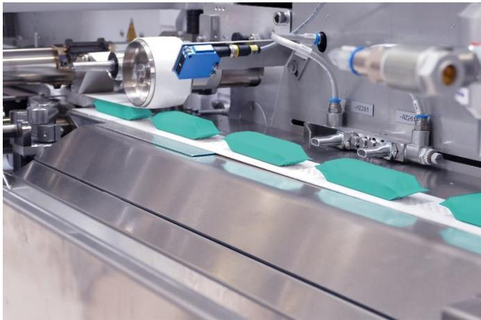
Photo 2: Theegarten-Pactec has developed the ideal solution for heat sealing paper-based packaging - in the high-performance range. This enables an impressive output of 90 m/min to be achieved on the FPC5. This corresponds to 600 sizeable 40g chocolate bars per minute.
