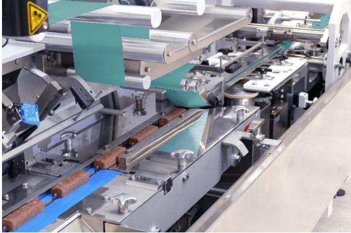
Photo 1: Theegarten-Pactec has refined its FPC5 - a modular high-performance packaging machine for bars in flow packs - so that it can now process paper-based packaging materials.
