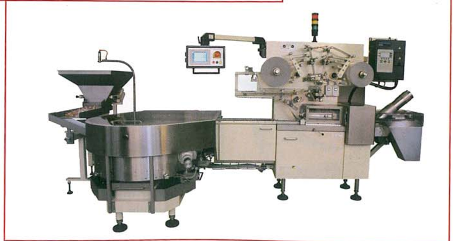
Theegarten-Pactec's FPL horizontal high-speed wrapping machine for lollipops in flow packs, can wrap up to 700ppm
